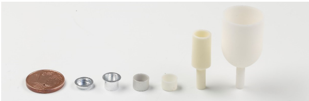
Fig. 1: By flowing different gases around the sample and using crucibles of different sizes (adapted to the application and question), a wide variety of tests can be carried out.
